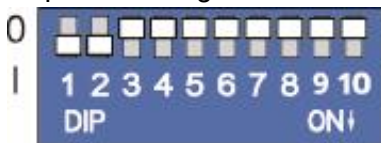
Figure 4: DIP switches (factory settings)
